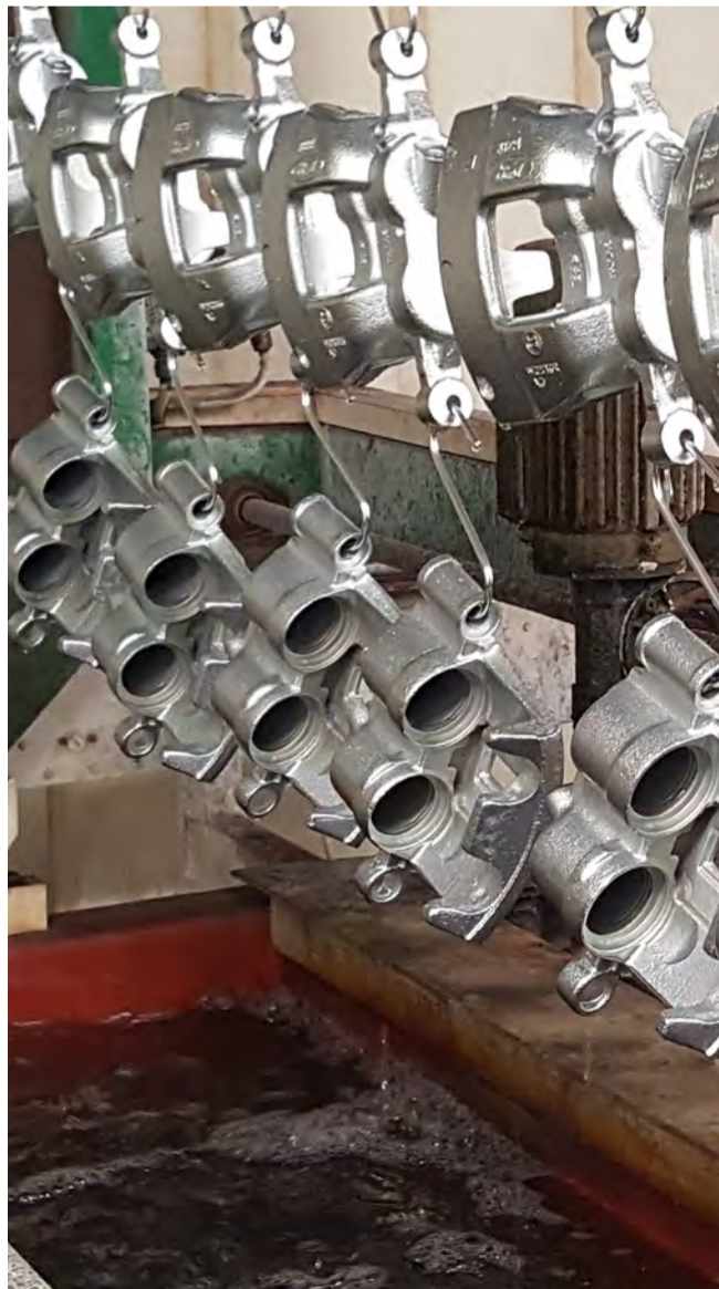
Galvanisation tank at Budweg. The tank is a closed system with no access to public sewage.
